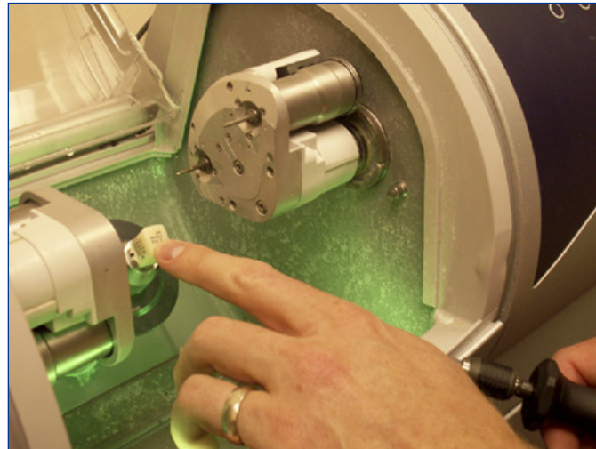
A block of ceramic material is placed in the milling machine. Rotating drills carve the material according to the instructions from the CAD/CAM system.
