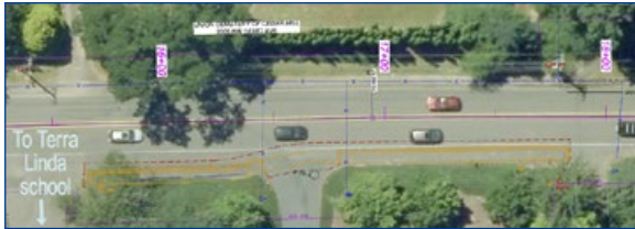
The new sidewalk section on 143rd will be next to the roadway but will be separated by a curb.
